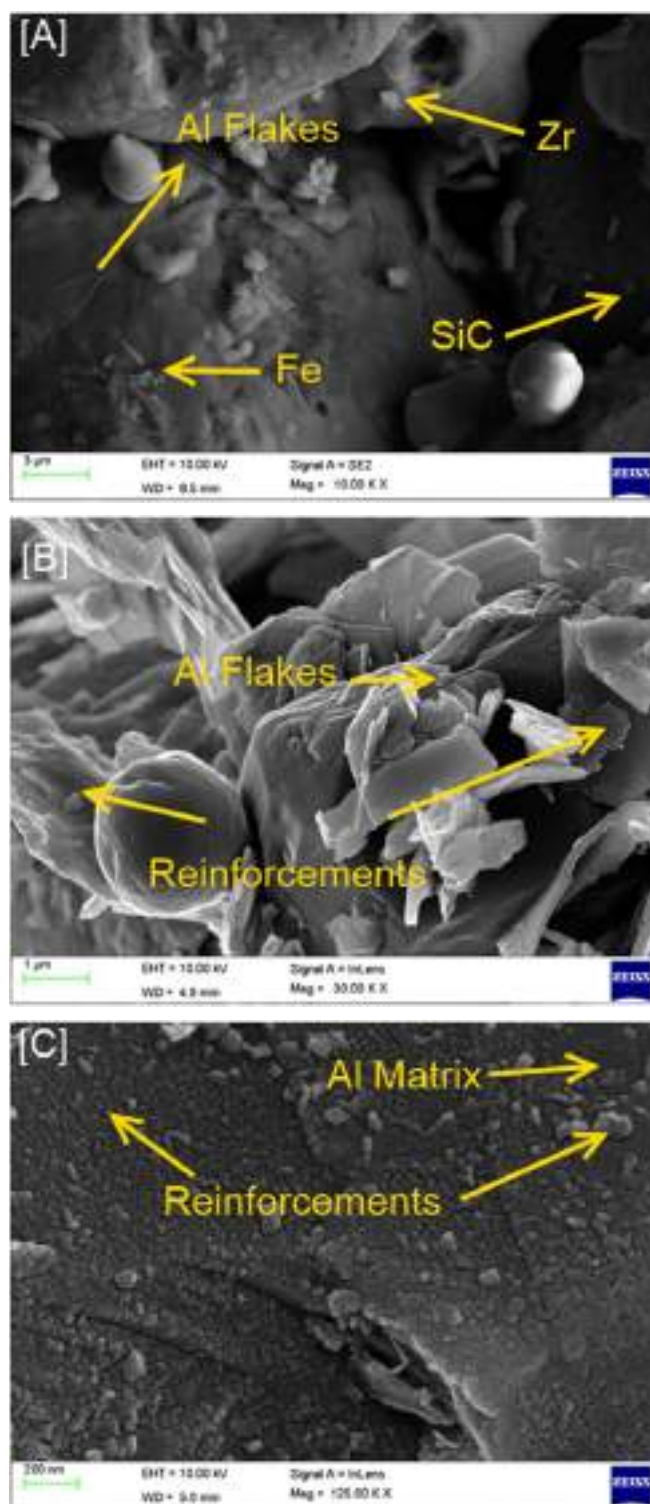
Figure 2. High Resolution Field Emission Scanning Electron Microscope (FE-SEM) image of Al-10Fe- 10SiC- 10Zr hybrid composites.
