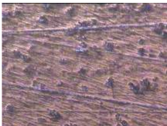
Fig. 16. Microstructure of welded area of EN 24.
