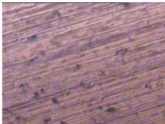
Fig. 15. Microstructure of welded area of EN 9.
